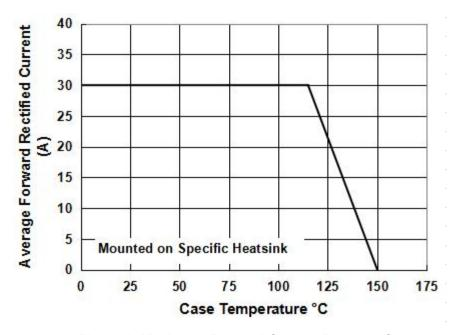
**Figure 1. Maximum Forward Current Derating Curve**
